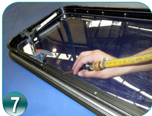
7 Clean window from aluminum swarf by blowing away with compressed air.
