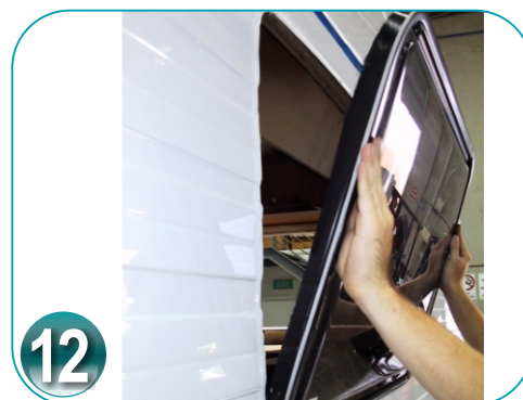
12 With the bottom of the window in place, gently push the top of the window in position in the opening.
