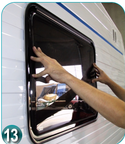
13 One person needs to hold window from the outside of the van until a second person starts reinstalling the clamping to the window from the inside of the van. Clamping must be reinstalled in exact position for the holes to match up.
