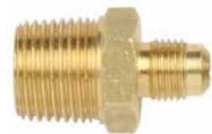
GAS ADAPTOR 1/2" MALE BSP X 5/16" SAE MALE FLARE 042580
