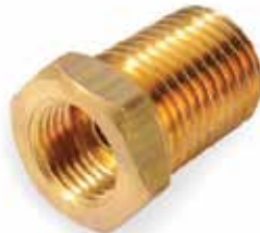
NO 62 - 1/4" MALE BSP X 1/4" FEMALE UNION 004033 Used to convert copper pigtailed with dual/changeover regulators. For use with single OPP regulators less POL.
